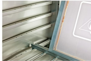
Bottom rail with inclination and leveling adjustment
